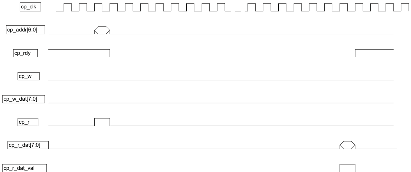
Figure 2-11. BB Control Plane Single Read Transaction
