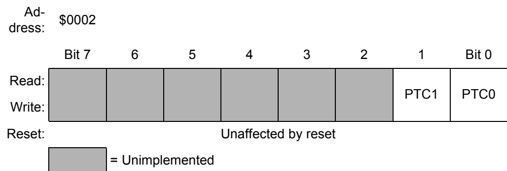
Figure 14-8. Port C Data Register (PTC)
