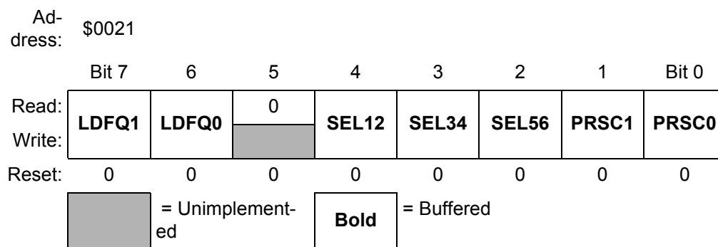
Figure 9-36. PWM Control Register 2 (PCTL2)
